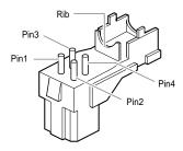
Connect the cable of the control cable, whose covering is stripped, to the Auto Iris Lens Connector as shown below.
